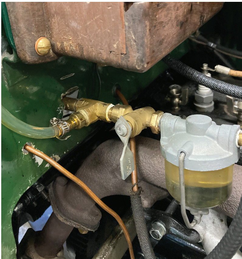
↑ Well known Florida car restorer Brad Hindall, impatient with trying to get an accurate measure of fuel in tank of his 1915 S-2 touring car, devised a simple sight-gauge that can be checked under the hood. By adding a clear plastic tube to the fuel tap, and securing it well over the wooden coil box, a driver can see at a glance exactly how much fuel remains.
