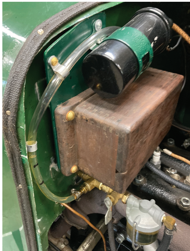
↑ Well known Florida car restorer Brad Hindall, impatient with trying to get an accurate measure of fuel in tank of his 1915 S-2 touring car, devised a simple sight-gauge that can be checked under the hood. By adding a clear plastic tube to the fuel tap, and securing it well over the wooden coil box, a driver can see at a glance exactly how much fuel remains.
